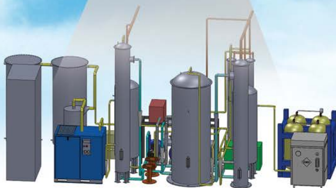
CMU-CBG system (Water Scrubbing Process)
